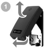
Pull bottom edge of reader module away from the backplate, and lift up.
